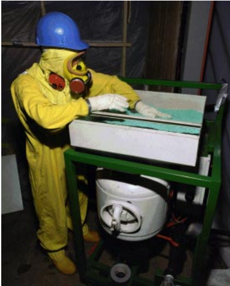
Figure 2. Portable pneumatically powered feed unit.
