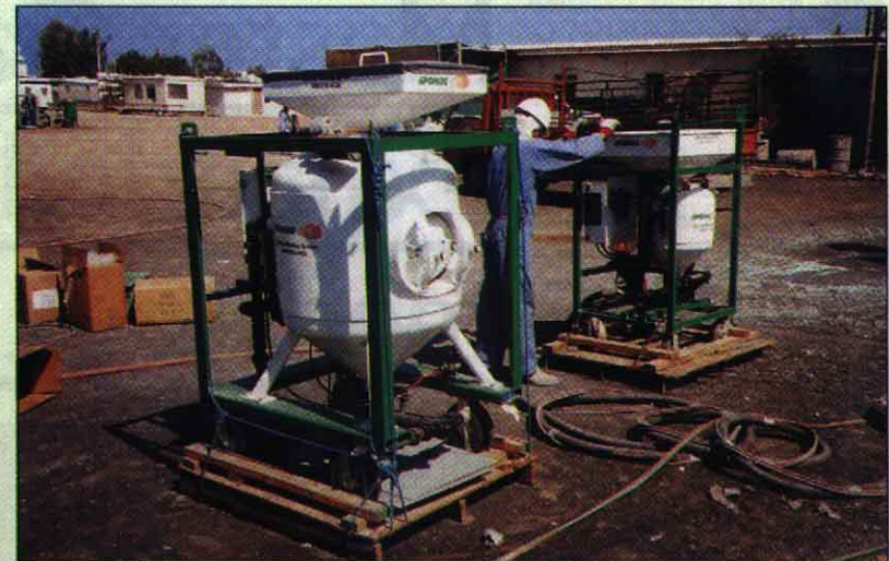
Sponge-Jet Feed Units are available in 280 and 85 litre capacities
